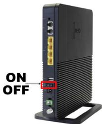
1. Turn OFF router using ON/OFF button on back of the device as shown on the image.
